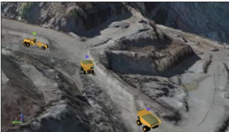
Using HAULSIM, our client could model the impact of congestion at critical areas in their mining circuits. Comparisons between the calibrated Discrete Event Simulation model and the models with the improvements indicated the impact of those changes on the bottom line. Specifically, our client inputted the following targeted data from their mine to generate realistic simulations on each improvement initiative to validate assumptions:
