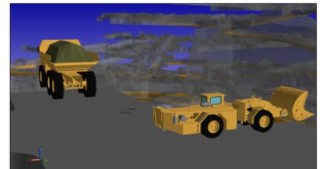
Each scenario was modelled on top of the base simulation to show the effects on total system productivity as the mine developed over a 3 year period. Along with this, quantifiable data was used to simulate the most cost effective strategy to improve equipment interactions and reduce overall truck travel time. Consequently, the site could effectively plan with full understanding of the outcome.
